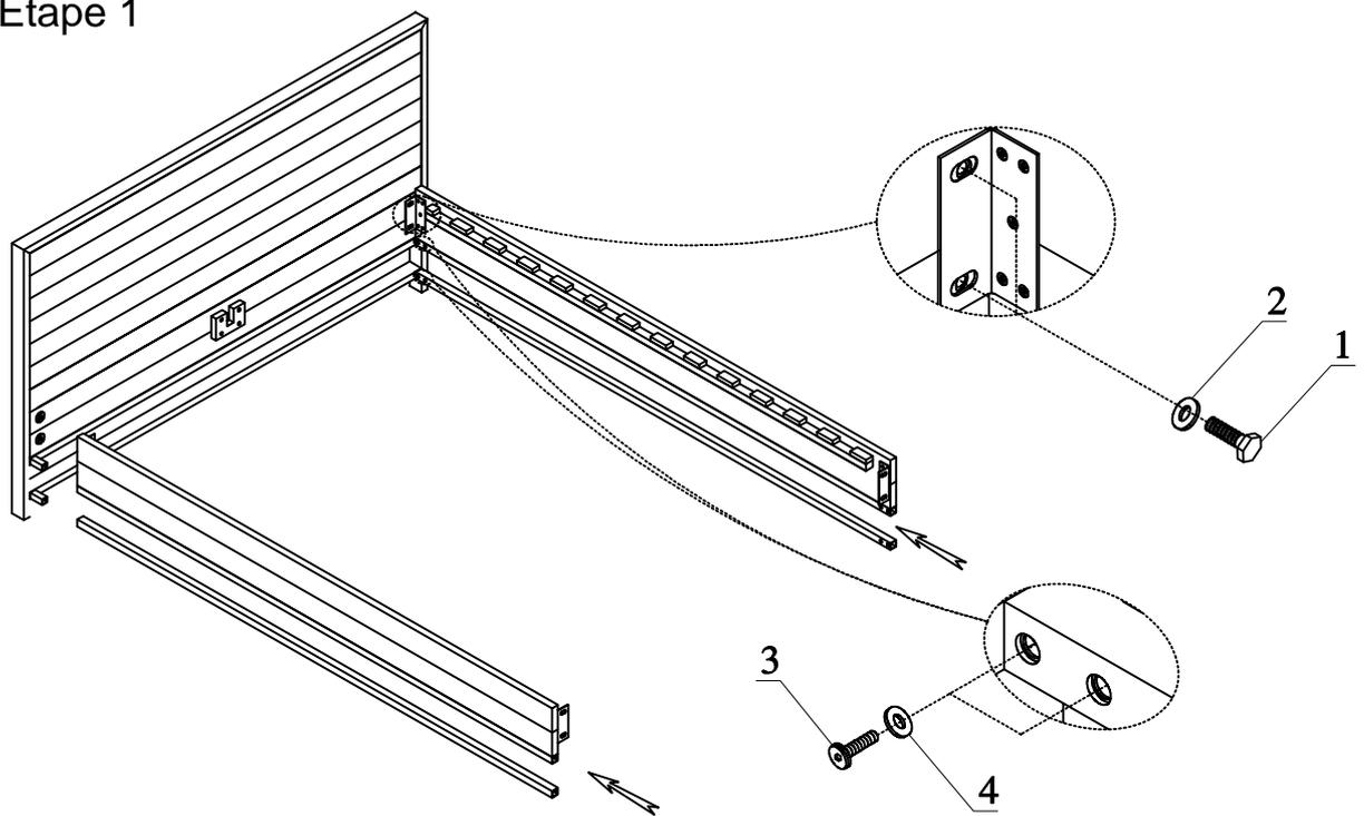
Please put side rails and slats on right position. Ensuring everything is aligned before tightening the bolt and screw.
